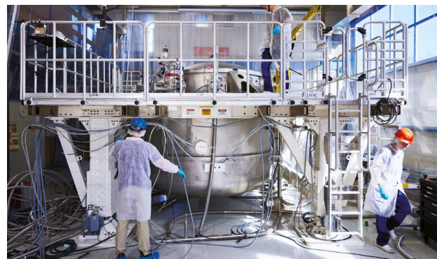
The METIS cryostat in the assembly support frame (in Buchs, Switzerland), being prepared for thorough testing before shipping to the NOVA AIT facility in Leiden. © ETH Zurich.
