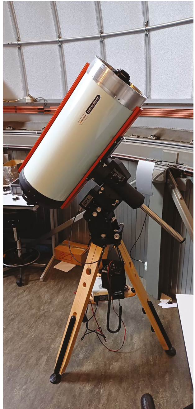
Proto-NUX assembled (without the replaced optics yet) at the UvA for testing.
