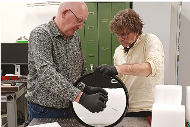
Hans Ellermeijer (UvA; left) & Rik ter Horst (NOVA; right) dismantling the mirror of proto-NUX so it can be recoated with a NUV reflective coating.
