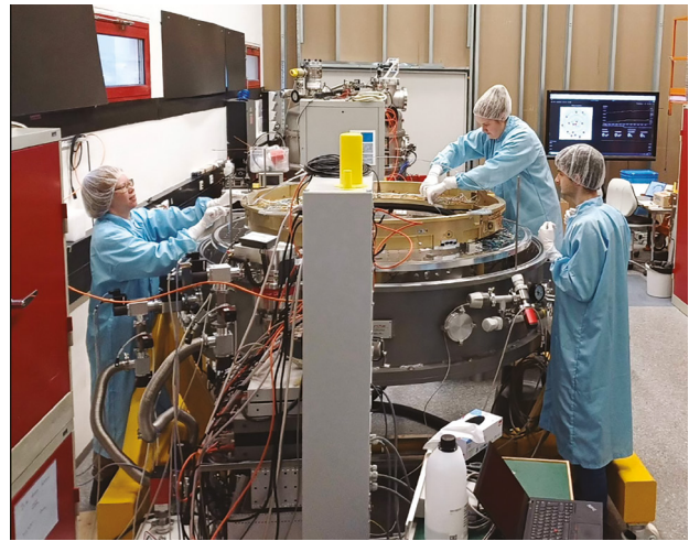
The MICADO pupil wheel mechanism, placed into the test cryostat at MPE for testing in March 2024.
