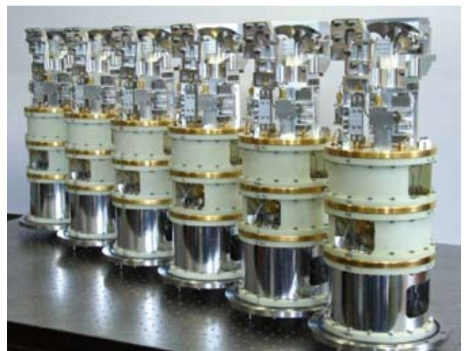
Figure 3.1: First six prototype ALMA Band-9 cartridges manufactured under ESO contract following NOVA funded instrument R&D in Phase-1.
