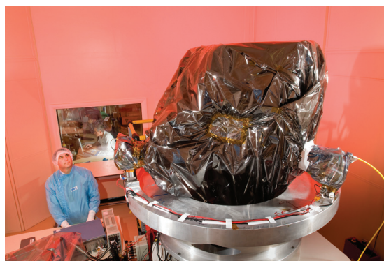
MIRI in the vibration test facility during the Flight Model AIV testing at Rutherford Appleton Laboratory in 2010.
