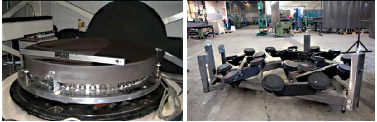
Figure 5.9: Left: AM1 under test at AMOS, the manufacturer of AM1. Shown is AM1 after its spherical lapping. In its final shape, AM1 will be an 1.7-meter aspherical mirror with a standard aluminum coating. Right: the support for AM1, manufactured at Boessenkool, in Almelo. This is the support without surface protection.
