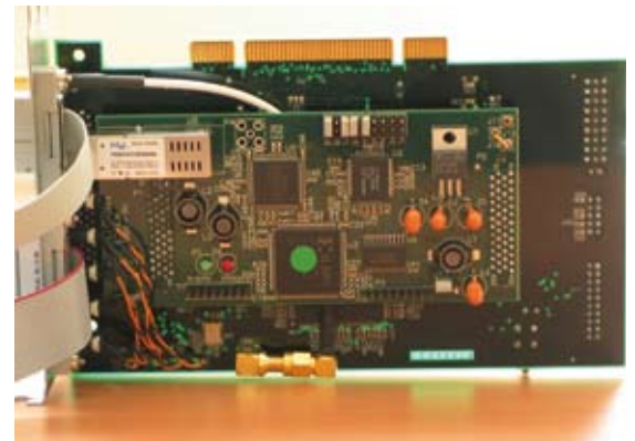
Fig. 5.7: The PuMa Interface Card (PiC) is the hardware component that connects PuMa-2 to the WSRT. It takes the optical, digital signals supplied and synchronizes and reformats them in a format suitable for subsequent recording. It is built around the PCI 9080 interface chip from PLX Technologies, and Altera ACEX FPGA. The card also has a daughter board (shown) to de-multiplex serial data from the Tied Array Adder Module. Board control, error detection, synchronization and status monitoring are basic tasks done in the FPGA. The PCI interface is used to communicate with the upper layer application software. The board and associated software were developed principally by Ramesh Karrupasamy (NOVA PhD) with able assistance from the staff in the Digital Laboratory at ASTRON and initial outlines from Stappers.
