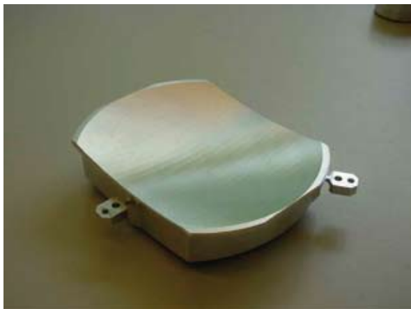
Fig. 5.12: MIRI Mirror Engineering Qualification Model (front and rear). Note the lightweighting of rear of mirror.
