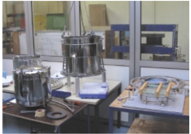
Fig 16: Parts of the OmegaCAM cooling system at the ESO workshop before integration. From left to right: inner liquid nitrogen tank, cryostat vessel, and heat exchanger.
